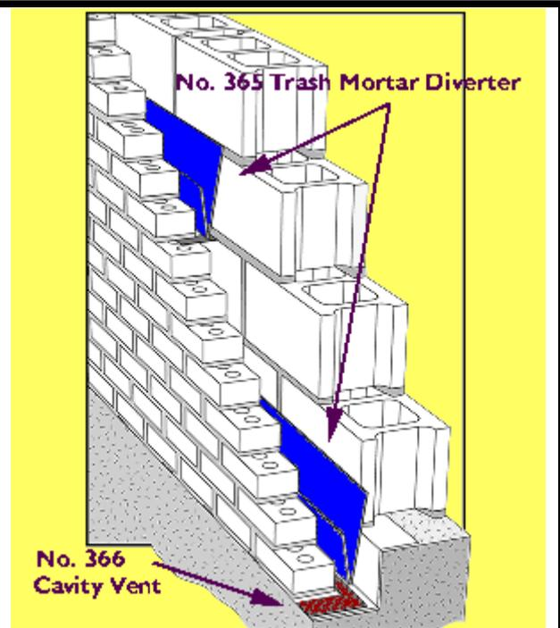
**Installation:** Insert Mortar Diverter into the cavity with "V" pointed in a downward position with the short edge to the outside of the building. Overlap the ends approximately 1" (25 mm). Field fabricate with a common utility knife.
