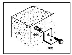
**TEST CONDITIONS:** The following chart is based on the average of many physical tests under proper conditions. (To obtain maximum load of insert machine bolt thread engagement must be at least 75% of the depth of the threaded hole. Use either bolts or threaded rods when attaching fixtures to the inserts.)
