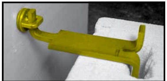
Stainless Steel Pos-I-Tie® Stone Anchors: Available 3/16" or 1/8" thick. Specify length, width, and bend type (Split-bend shown above, straight bend, or pin type available).
