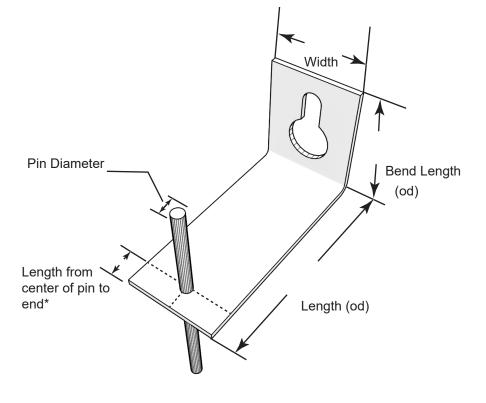
\*Pins are available loose or welded in place.
