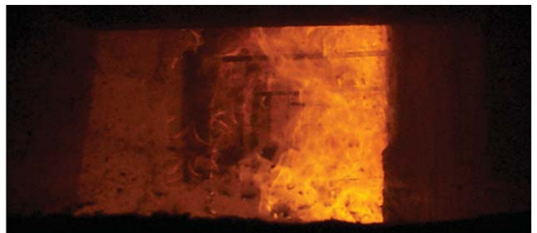
Fire Exposure Inside ASTM E119 Furnace
