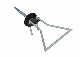
The Heckmann Composite Resin Thermal Clip, when attached to a Heckmann Pos-I-Tie® barrel, will provide a pullout load exceeding 500 pounds failure. This test was a pullout of the wire tie from the thermal clip only. It did not take into consideration the pullout of the threaded screw from the backup. Additional tests of the Pos-I-Tie® system with different wall conditions can be found on our website at www.heckmannnanchors.com.
